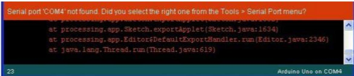
The clue is at the top here, it probably means that your board is not connected at all, or the drivers have not been installed (if necessary) or that the wrong serial port is selected.
