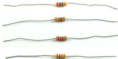
220 \Omega Resistor (red, red, brown stripes) 1
