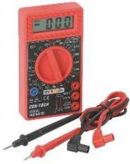
A multimeter or a multitester, also known as a VOM, is an electronic measuring instrument that combines several measurement functions in one unit. A typical multimeter can measure voltage, current, and resistance. Analog multimeters use a microammeter with a moving pointer to display readings.
