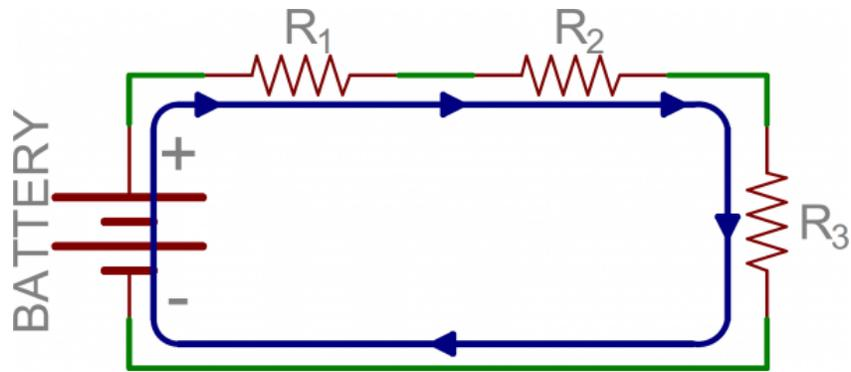
There's only one way for the current to flow in the above circuit. Starting from the positive terminal of the battery, current flow will first encounter  $R_1$ . From there the current will flow straight to  $R_2$ , then to  $R_3$ , and finally back to the negative terminal of the battery. Note that there is only one path for current to follow. These components are in series.
