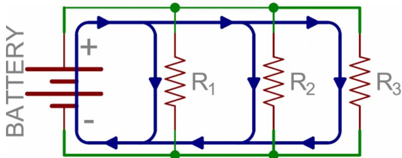
From the positive battery terminal, current flows to  $R_1$ ... and  $R_2$ , and  $R_3$ . The node that connects the battery to  $R_1$  is also connected to the other resistors. The other ends of these resistors are similarly tied together, and then tied back to the negative terminal of the battery. There are three distinct paths that current can take before returning to the battery, and the associated resistors are said to be in parallel.
