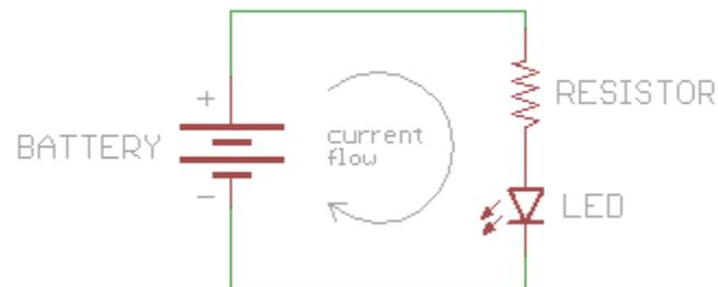
**This circular path, which is always required to get electricity to flow and do something useful, is called a circuit.** A circuit is a path that starts and stops at the same place, which is exactly what we're doing.
