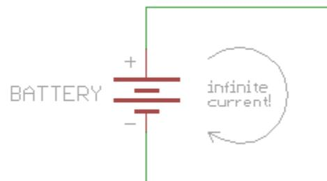
This seems like the best possible circuit, so why is it a bad idea? Remember that electrical current wants to flow from a higher voltage to a lower voltage, and if you put a load into the current, you can do something useful like light up an LED.
